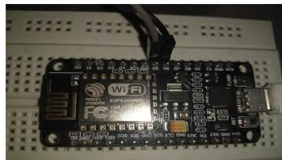
Fig3.4 wifi module-ESP8266MOD connection
